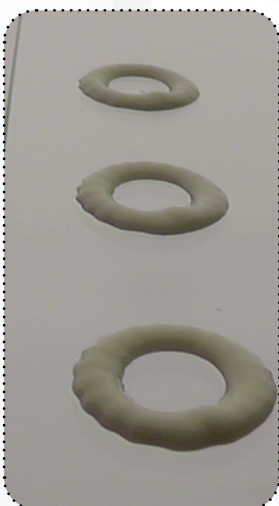
Fig. 3: Minimum line widths of up to 0.8 mm are already feasible today (Image: perfecdos GmbH)
